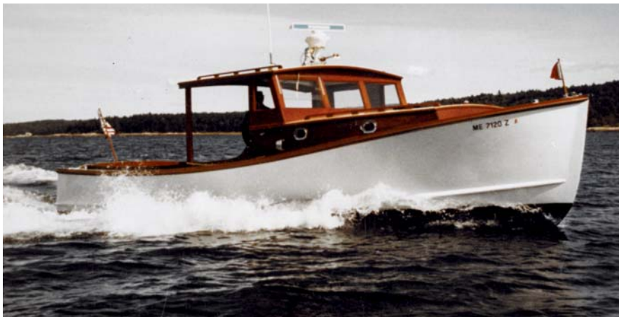
The Stanley 36 Gambol , which was built in the 1980s, was one of the first Stanleys built as a pleasure boat. The previous ones had been used for lobstering. Williams modified the lines to raise the sheer.
